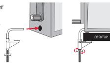
2 Holding the handle still, turn the pencil point options knob to adjust the sharpness.
